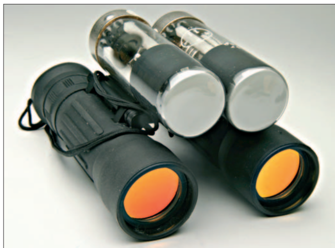
● An interesting instrument? No, it's not a mock-up of a twin tube bino-oscilloscope! Instead, it's Tex G1TEX's way of demonstrating the possibilities with the 1CP1/DH3-91 miniature oscilloscope tube, shown photographed with a pair of 10 x 25mm binoculars.
