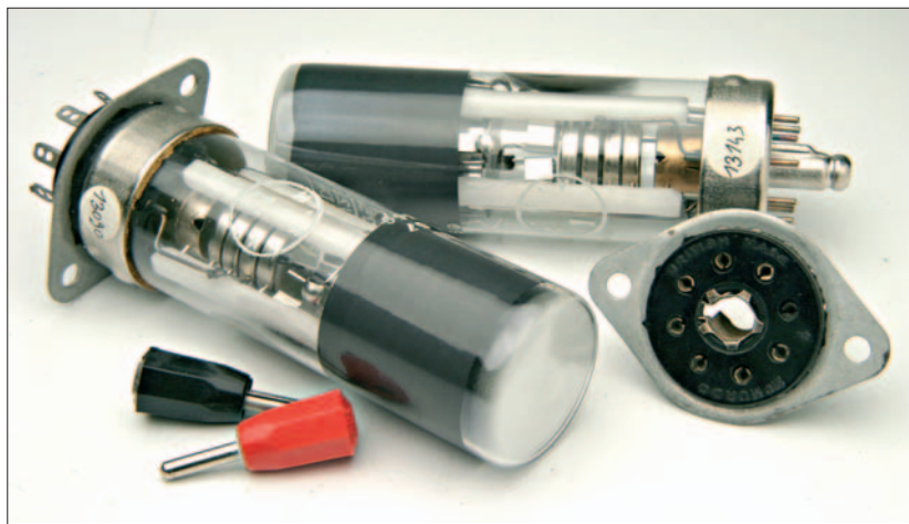
● Fig. 1: Small but useful! The 1CP1 (DH3-91) one inch oscilloscope tube is small - as indicated by the wander plugs and B8G base - but it's still a full functioning display device. The proposed Radio Basics 'scope project will use this c.r.t. (see text).
