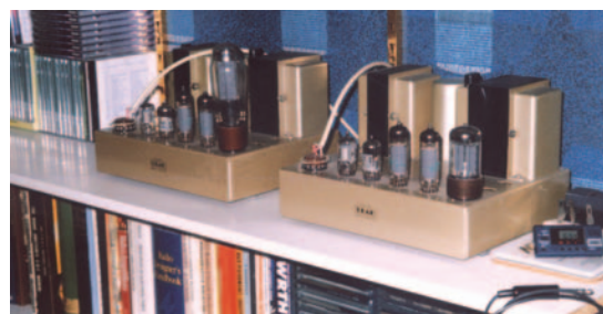
● Phil Cadman G4JCP doesn't just write about valves - he enjoys using them! This photograph shows a pair of Leak TU/12 Plus amplifiers. They're Phil's pride and joy and are a variant of the Mullard 5-10 circuitry (see text).
